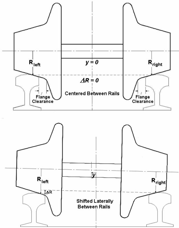
Figure 2 - Example Rolling Radius Difference Curve
