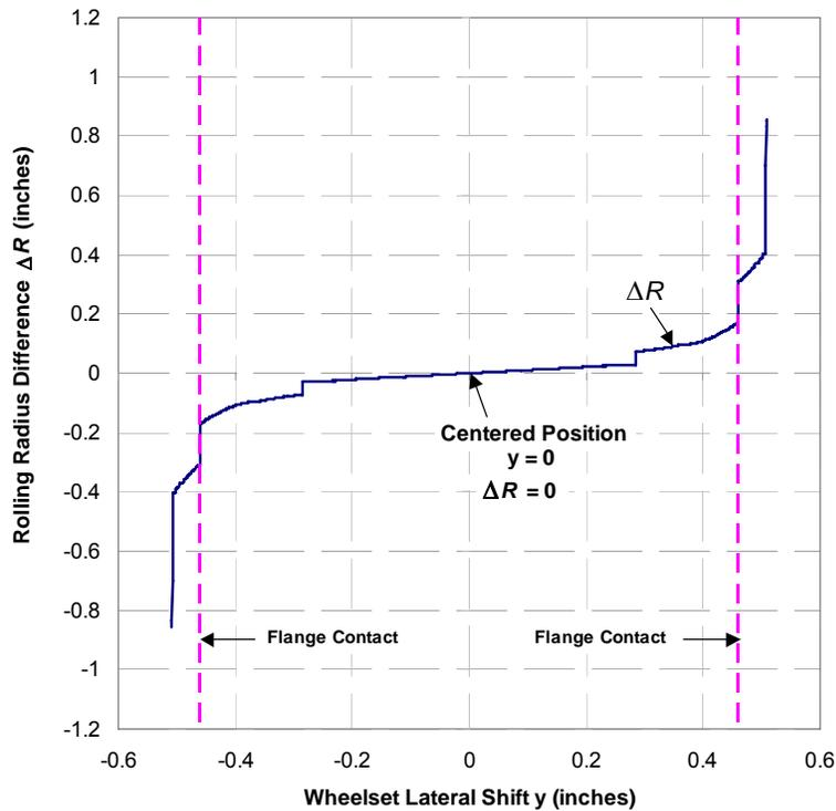
**Figure B1 – Example Rolling Radius Difference Data**
